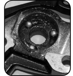
29. Apply a high-strength thread-lock such as Loctite 272 to the drive cam threads.
