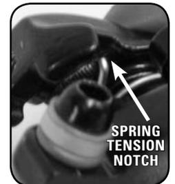
31. Install the torque arm, aligning the spring leg with the spring tension notch on the back of the torque arm. When engaged correctly, the spring adjuster screw will be driven against the spring leg on the back of the torque arm. Press the torque arm onto the flats of the drive cam shaft. Make sure the arm is fully seated and hold firmly with your thumb.
