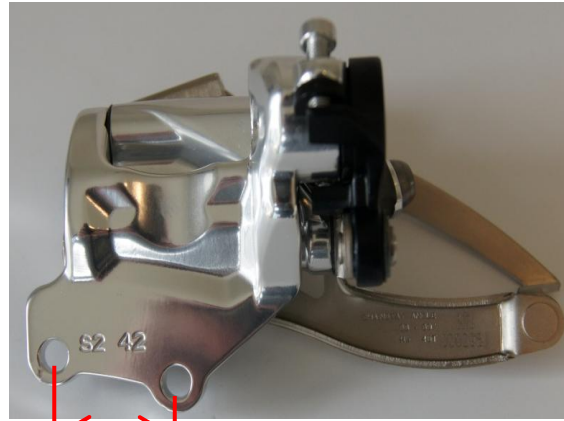
Measure eye to eye. S2 = 22,50 mm.
