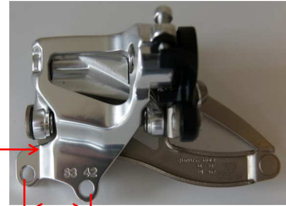
Measure eye to eye. S3 = 22,50 mm. NOTE: Plate level difference . (approx. 5 mm)
